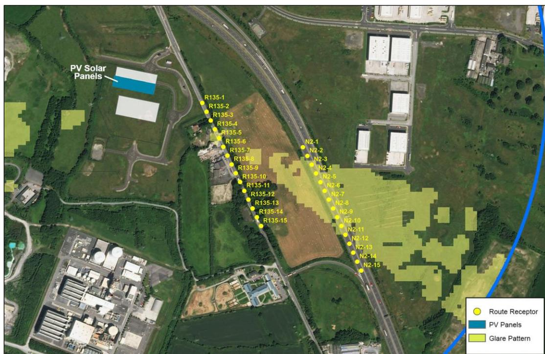
**Figure 3:** Route receptors identified within 1km of the proposed solar PV development that intersect with the predicted glare pattern.
